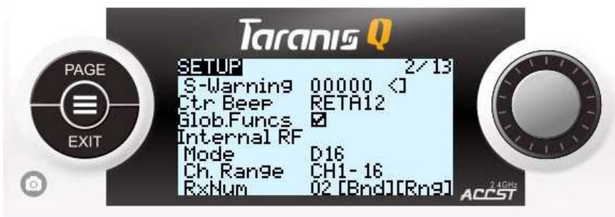
Press and hold BIND button on your receiver, power it up. Release BIND button. Power off the receiver. Press "EXIT" on the radio to leave the BIND mode. Power on your receiver again. This time the green led on the receiver should be constantly lit indicating that there is a connection to the radio.
