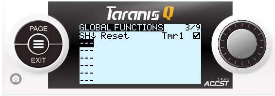
*Interpretation: global function of line1 would act as Timer1 reset to the max. desired time set in "SETUP"->"Timer1" model menu when you pull SH momentary switch towards you (max. value).*
