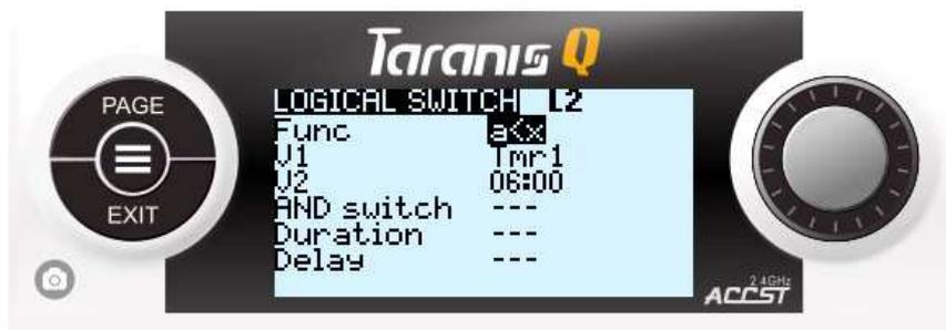
*Interpretation: logical switch L2 would be activated if: Tmr1 current countdown time is less than the max. desired time of of the timer1. So, this Logical Switch would work all the way from 05:59 and down to -xx:xx time unless we would reset our timer1 to 06:00.*
