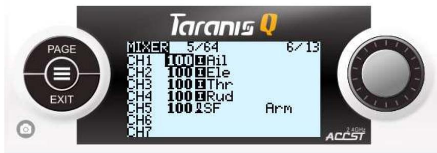
*Interpretation: CH5 of the receiver would receive 100% (full range) of SF switch input (-100 (negative endpoint) signal at SF switch at down (far from you) position and +100 (positive endpoint) signal at SF switch at up (close to you) position).*
