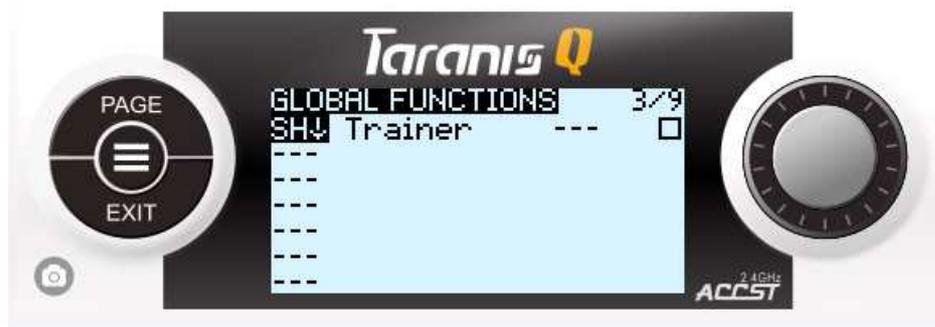
Select next field to the right and set the value to "RESET" and third field value to Tmr1. And put a checkbox in the next field. Press "EXIT" to return exit the line edit.
