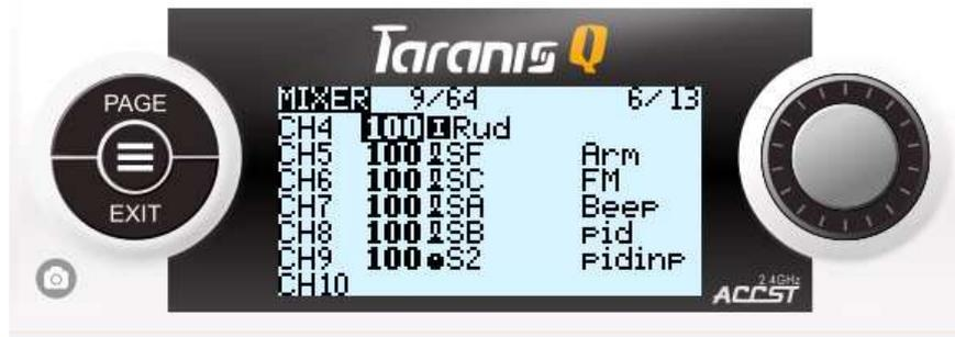
*Interpretation: CH9 of the receiver would receive 100% (full range) of S2 pot input (from -100 (negative endpoint) signal at S2 full to the left to +100 (positive endpoint) signal at S2 full to the right. With 0 (center) signal at center detent point).*
