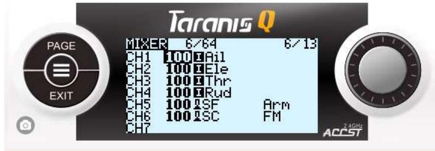
*Interpretation: CH6 of the receiver would receive 100% (full range) of SC switch input (-100 (negative endpoint) signal at SC switch at upper position, 0 (center) signal at SC center position and +100 (positive endpoint) signal at SC switch at down position).*
