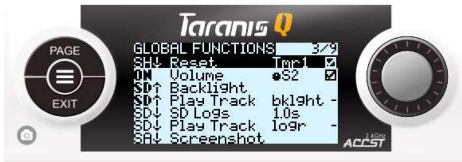
Highlight the first empty line, press "ENTER" and move SH switch towards you to get "SH ↓" reading, press "ENTER" again to save this value.
