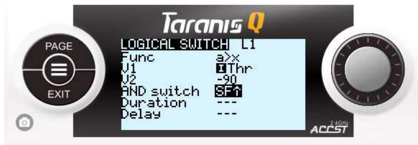
*Interpretation: logical switch L1 would be activated if: Thr input is more than -90 and if SF switch (ARM) is at furthest from us (minimum, ON is you set it right in the F3 board) position.*
