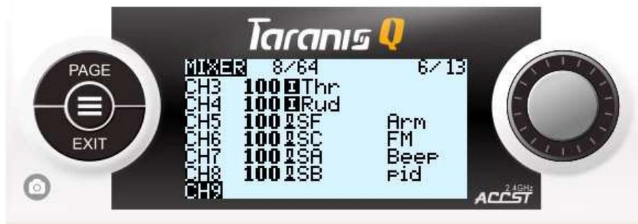
*Interpretation: CH8 of the receiver would receive 100% (full range) of SB switch input (-100 (negative endpoint) signal at SB switch at upper position, 0 (center) signal at SB center position and +100 (positive endpoint) signal at SB switch at down position).*
