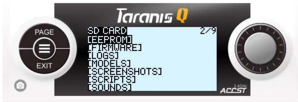
with the right rotary dial navigate to "FIRMWARE" folder, press enter, navigate to the FW file you have here, long press "ENTER" (center rotary dial press) and select Update bootloader. Now, you have your bootloader up to date and with the version corresponding to the radio FW file. Hit "EXIT" several times to get back to the main flight screen.
