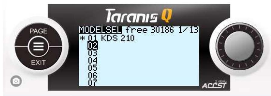
*\*note: if you would create a new model – it would automatically have 1<sup>st</sup> 4 channels in the order as you have stated in "RADIO SETUP" menu (in my case AETR). That is why we needed to set this channel order in "RADIO SETUP" according to our preference. The default model that you have on the radio from the factory has another 1<sup>st</sup> 4 channels order. I prefer to delete such models and create a new one.*
