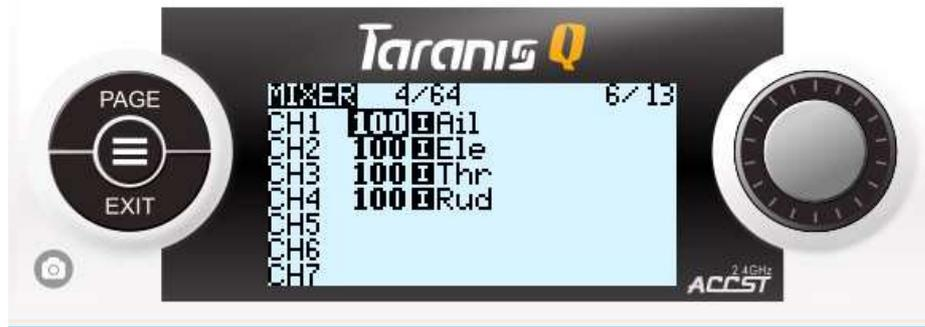
This screen is a core of all model channel behavior. Whenever we want to make any changes to the way the channel outputs are functioning – we would have to create or edit our mix for the corresponding channel. Now, if you have followed this document – you see the same mixes as shown on the screenshot. Only 4 mixes for 4 1<sup>st</sup> channels in AETR order. This shows us that first 4 channels are already working... Let me explain how it interprets. Let's take the first line:
