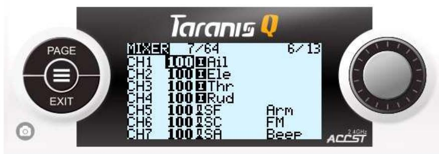
*Interpretation: CH7 of the receiver would receive 100% (full range) of SA switch input (-100 (negative endpoint) signal at SA switch at upper position, 0 (center) signal at SA center position and +100 (positive endpoint) signal at SA switch at down position).*
